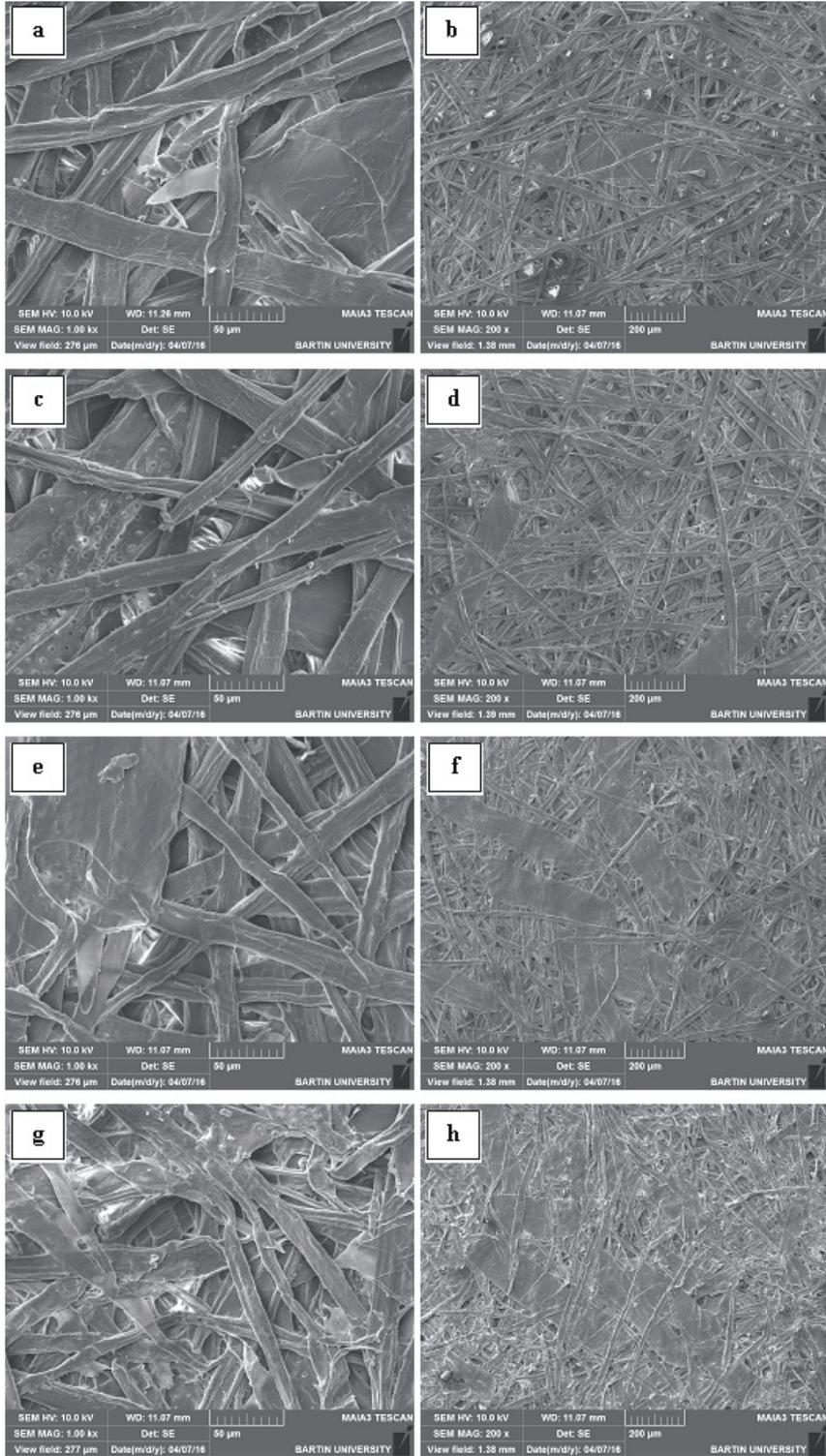
**Figure 7.** FE-SEM handsheet micrographs of each fractionation of European aspen kraft pulp: a, b) R30; c, d) R50; e, f) R100; g, h) R200.
