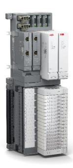
Select I/O: Modular, single point, late binding, Ethernet I/O solution that can be digitally marshalled into the ABB Ability™ System 800xA architecture
