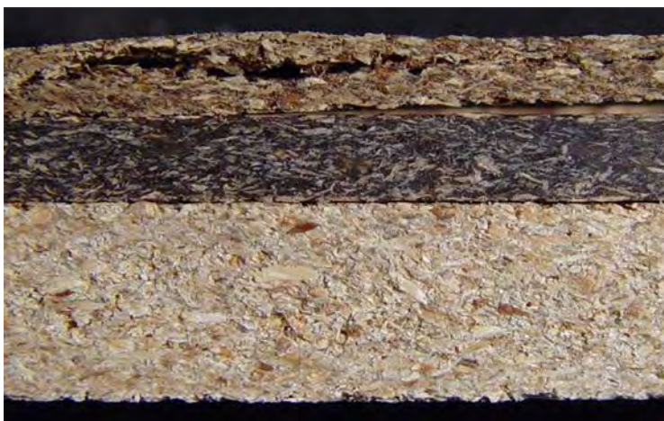
Fig. 8. Comparison of composite panels. Top panel consists of 50:50 mixture of DDGS: PW subjected to fast cooling. Note blistering and internal cracking. Middle panel consists of 50:50 mixtures of DDGS:PW subjected to slow cooling. Note absence of disruptive blemishes. Bottom panel is commercial PB locally purchased
