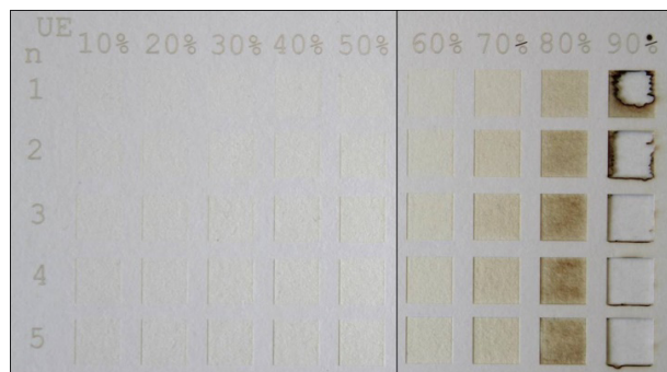
Fig. 3. Ablation of paper P2 using a peak fluence of 9.05 J/cm 2 . Different \Omega (here named UE) are shown on the x-axis, on the y-axis the number of transitions are increased.
