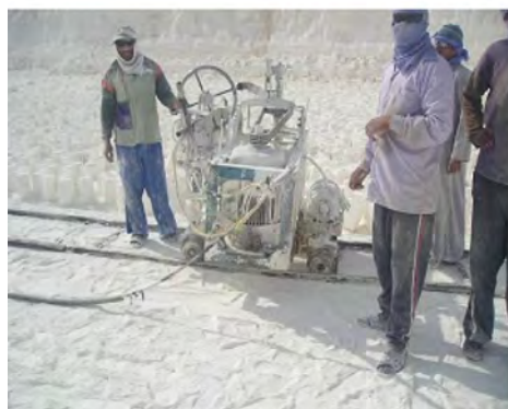
c- Cutting of limestone building blocks
