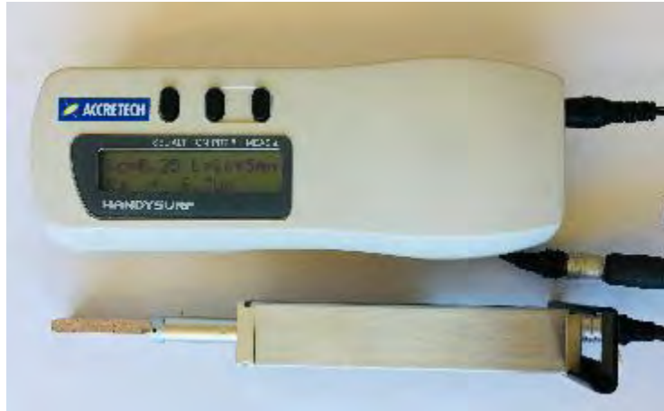
Fig. 3. The surface roughness measurement system
