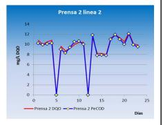
Figure 1: peCOD (blue) versus traditional method (red) for COD analysis at Diffusor Line 2.
