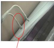
Deposit on second nozzle, created by the first nozzle
