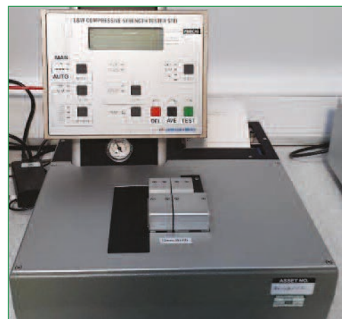
Figure 3. L&W Compressive Strength Tester STFI.
