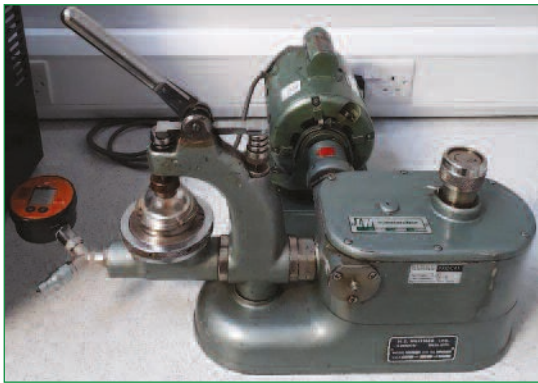
Figure 4. L&W Burst Strength Tester.
